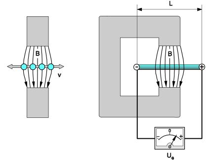
A voltage is induced in an electric conductor is moved through a magnetic field.
